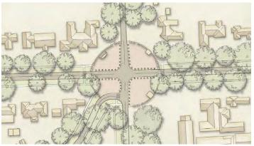
Solutions include signalizing the intersection to allow for pedestrian signals and adding north-south crosswalks, as well as removing the channelized right turn lanes.
