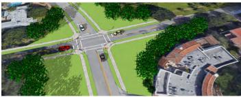
Adding crosswalks across all legs of the intersection and constructing a sidewalk along the northern side of Coral Way to the east of the intersection, will provide more visibility to pedestrians. A longer-term solution to remove the channelized right turns, or to add stop bars at each right turn lane, would limit pedestrian exposure and improve safety and accessibility.
